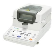
Halogen Light Heating Stainless Steel Chamber Temperature and time can be set The percentage of moisture content
